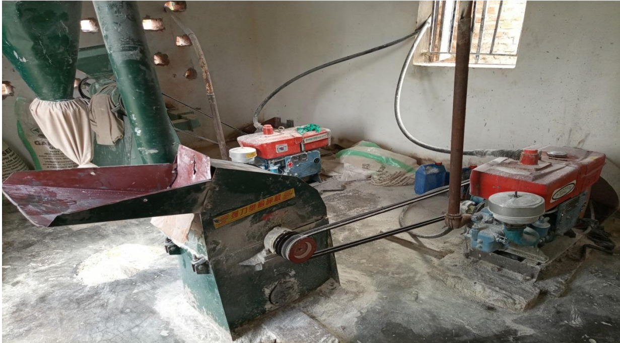
GAPSEC maize thresher, huller and miller machines installed for first class maize flour processing.
